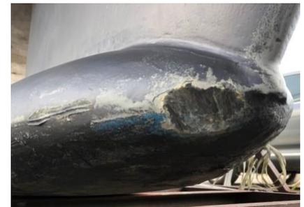
Figure 4: Lead keel impact - That should buff out!
